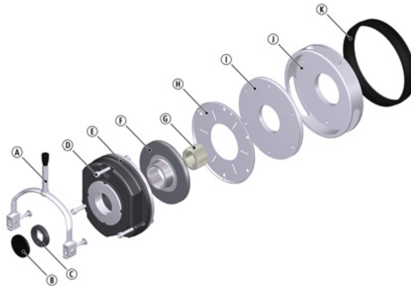
Fig. 34: Spring-applied brake INTORQ BFK458-06 to 25
