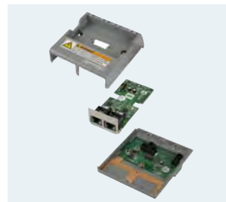
Function extension through optional module support for I/O and communication
